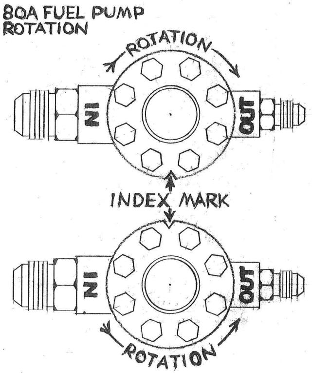
The 80A fuel pump will operate in a clockwise or counter clockwise rotation. The front cover of the pump must be orientated correctly for the desired rotation. On the outside diameter of the cover is a vee shaped notch. This notch must be alined as shown above for the required rotation. To change the fuel pump rotation, remove the 8 bolts from the pump cover and turn the cover exactly 180 degrees. Cam driven pumps turn clockwise and most belt driven pumps turn counter clockwise.
